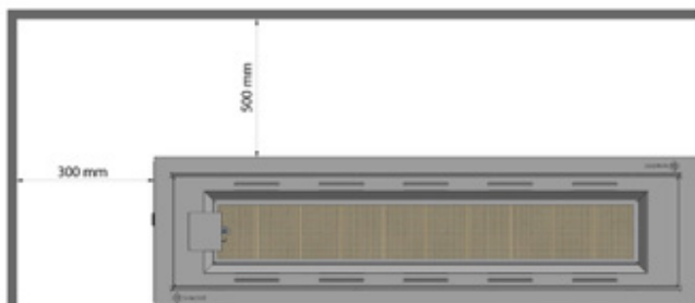
Fig. 3. Minimum free space from flammable materials / objects
