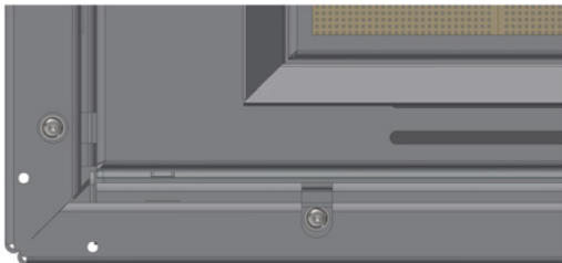
Fig. 9. Disassembling/Replacing of the glasses in PATIO HORIZONTAL
