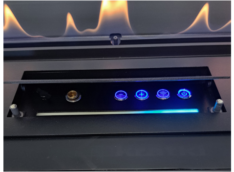
Fig. 9-11 Led strip in offline mode, there is about 25% fuel in the tank
