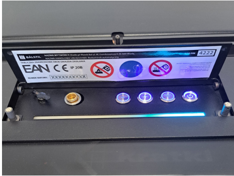
Fig. 9-10 Indication of approximately 25% of the fuel in the tank while the unit is online
